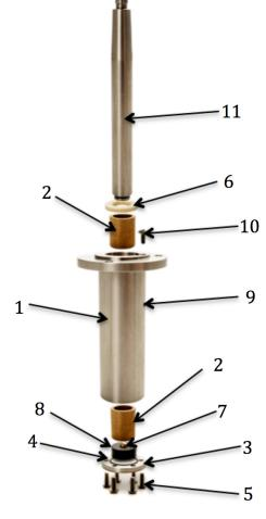
The bearing features an oil delivery system to keep the Oilite bushes lubricated and prevent them drying out. The bearing comes pre lubricated from the factory but the following procedure should be followed: The felt washer should be removed and then the M3 screw under the felt washer should be unscrewed and just a few drops of oil added. The oil will work its way down to the bottom bush and keep it sufficiently "oiled" allow time for air to come out.
